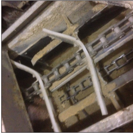
BEFORE: The old style of drag conveyor at the rice mill used bent welded-steel flights and UHMW paddles. Photos courtesy of 4B Components Ltd.
