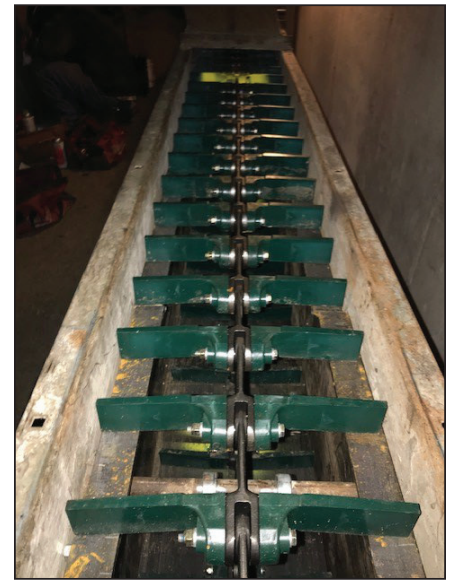
AFTER: Bolt-N-Go chain features nylon paddles bolted directly onto the chain without the need for welded-steel backers.
