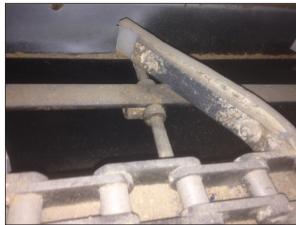
BEFORE: The old style of drag conveyor at the rice mill used bent welded-steel flights and UHMW paddles. Photos courtesy of 4B Components Ltd.
